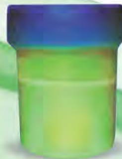
Sample of hydraulic fluid with FluidSafe additive at 0.015% under high-intensity blue light
